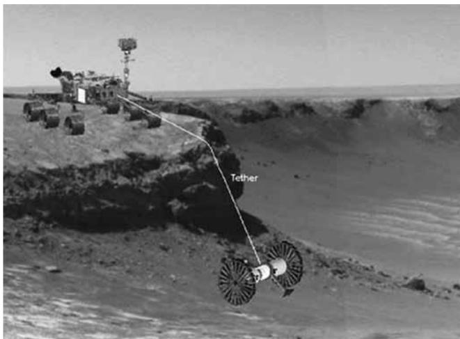
*Figure 3: A rover anchors itself on the rim, and a 2-wheel rover lowers itself down by paying out a cable. <http://www-robotics.jpl.nasa.gov/roboticImages/img811-414-browse.jpg>*
