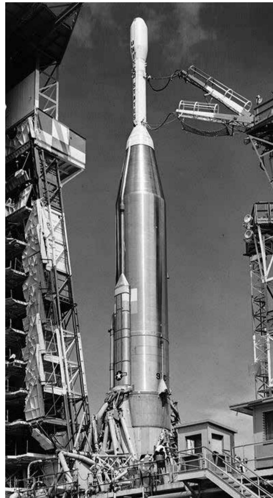
one on top could fire twice to slow it down to enter lunar orbit. The new Pioneers were the first lunar probes with a self-contained liquid-fueled propulsion system.
